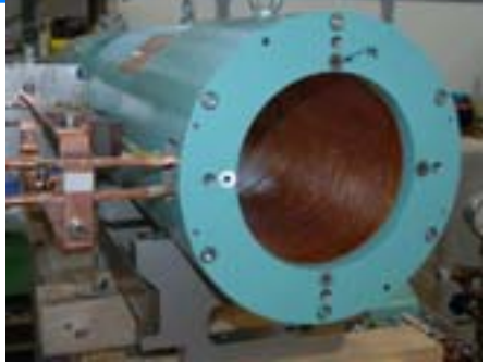
Gun solenoid (0.35T, A=80 mm, L=0.260 m)
